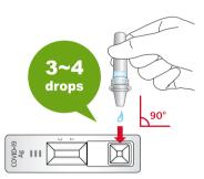
6 Invert the assay diluent tube and gently squeeze it to dispense 3-4 drops (90-150 $\mu\ell$ ) into a sample well on the device vertically.
