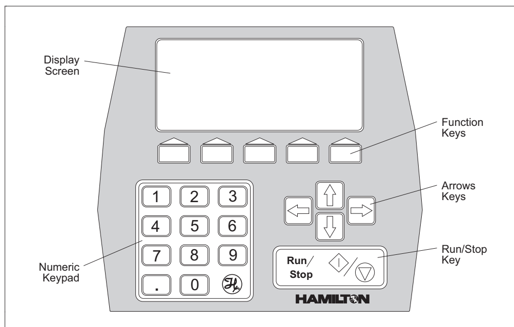
Figure 3-3 The Controller Unit
