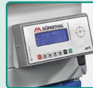
Exhaust air monitoring
