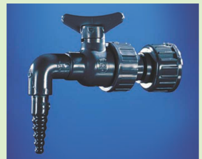
TKA Purified water outlet tap Made of plastic, angled. Connector R 3/4", coupling nut. Dimensions: 50 x 90 x 140 mm. No. 03.1401
