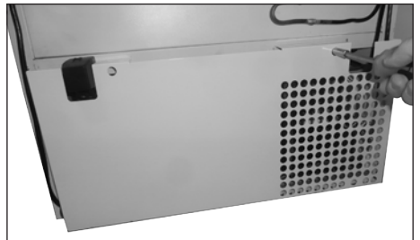
11. Fasten the cover with the 3 screws
