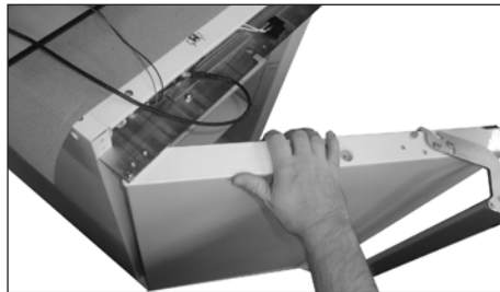
38. Re-locate the door on the cabinet in the new hingeside
