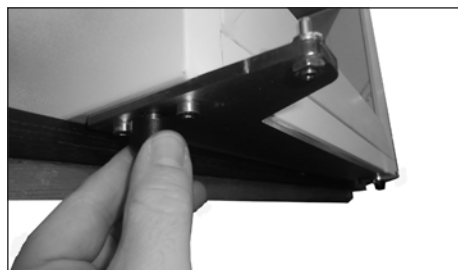
30. Remount and tighten the two front feet
