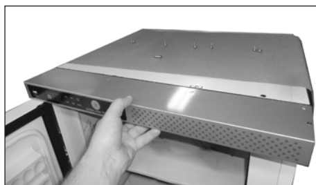
40. Carefully push the toppanel back into position
