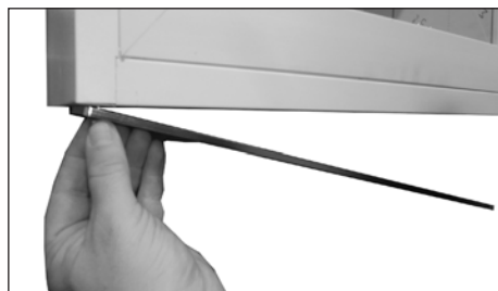
26. Loosen the screws in the opposite side and rotate the bottom door bracket
