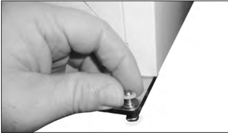
17. Go to bottom and remove the door pivot nylon washer
