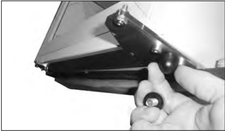
18. Remove the two front feet
