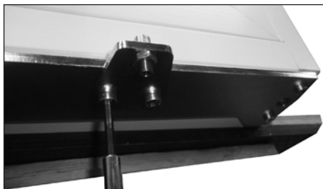
19. Remove bottom handlelock pin plate by loosening two screws (use 4 mm allen key)
