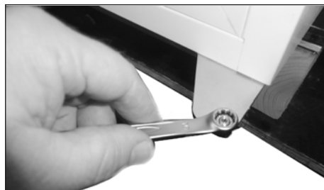
24. Remount and tighten pivot nut
