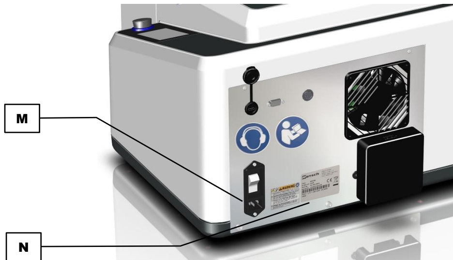
Fig. 14: Connecting to the power supply
