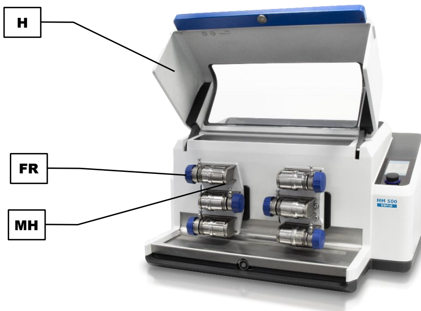
Fig. 24: Removing the grinding jar
